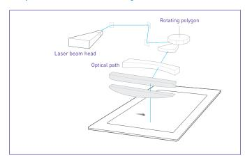
Fine line structure in a single scan enabled by KLA's field-proven LSO  $^{\text{\tiny{IM}}}$  technology.
