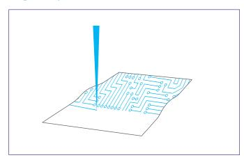
High depth-of-focus (DOF) for best line precision and uniformity on varying surface topographies.
