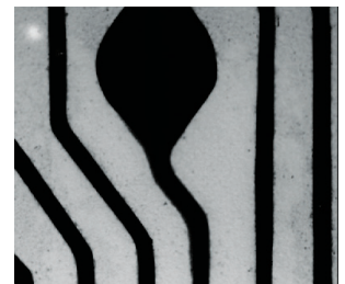
Open after 3D shaping. UV light image.
