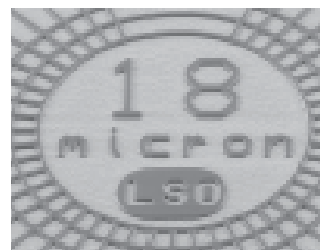
Fine lines/spaces of 18µm
