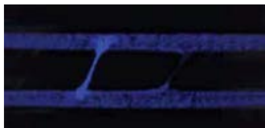
Blue light image - clear distinction between dust and fine short (dust is much brighter)
