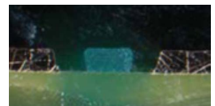
100μm solder dam, 40μm SM thickness on prepreg
