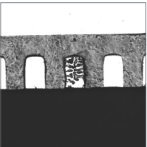
Bleed on Pad
